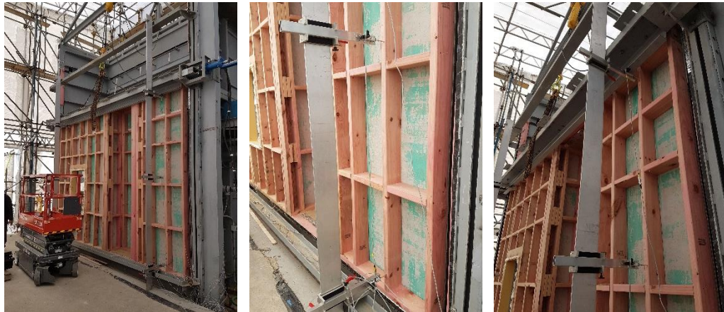
Figure 10: Photos of transducers on stud in field of wall (Stud 2)
