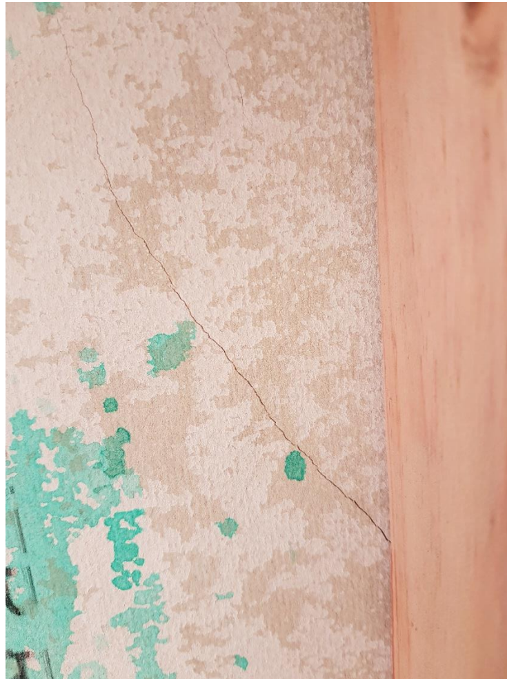
Figure 12: Crack in RAB board following ULS seismic testing on system
