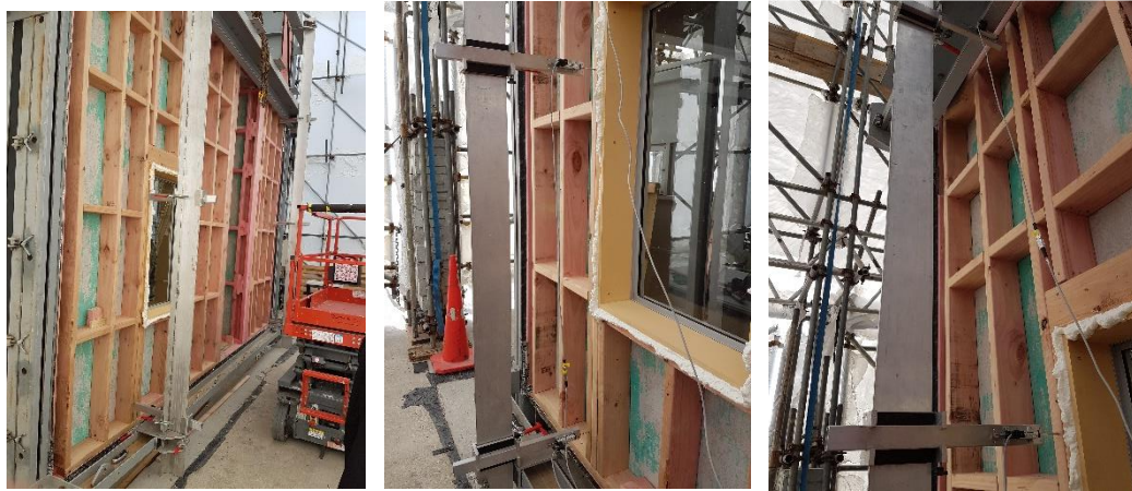
Figure 9: Photos of displacement transducers on stud beside window (Stud 1)
