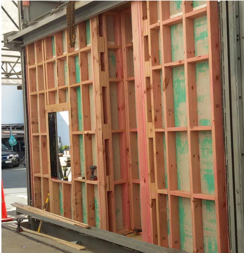
Figure 1: Sample under construction for testing showing dry-side
