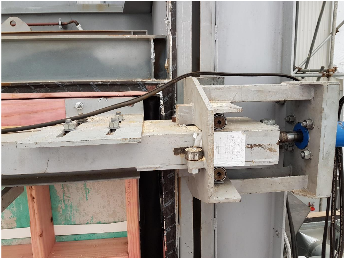
Figure 11: Top right hand corner of sample connected to the seismic ram via steel plates and bolts through the framing.
