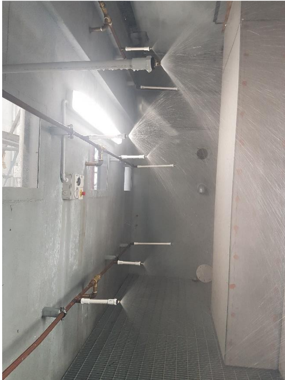
Figure 7: Water sprays on during static water test
